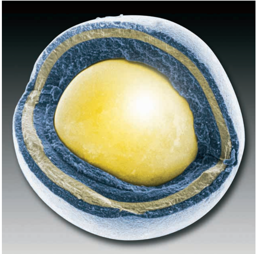
TRISO fuel particle. Source: Idaho National Laboratory.
