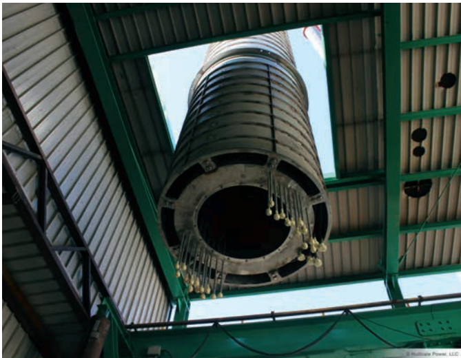
NuScale Power's full-length helical coil steam generator. © NuScale Power, LLC
