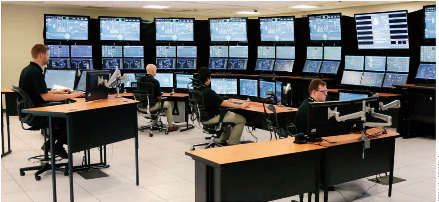
The NuScale Power Control Room Simulator is designed to simulate the operation of a 12-module NuScale power plant.
